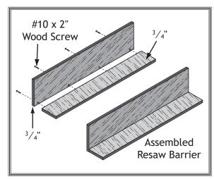
Figure 59. Shop-made resaw barrier.
